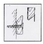
A hanger board may be fabricated using a 1x4, cut at a 45-degree angle. You may also cut a piece of wood that runs the length of the mantel shelf or use 2 blocks of wood that will be placed at either end of the mantel shelf. See above for measuring. Set the mantel on the length of wood or blocks. Use finishing nails on back side of legs (right underneath the back overhang of the shelf) to fasten to length of wood or blocks.
