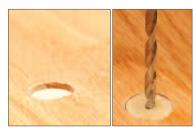
21. The 3/4" holes need to be plugged and glued with the included dowels. Check that the hole depth exceeds the dowel plug by about 1/16". Drill a 13/64" size vertical hole into the center of the dowel.
