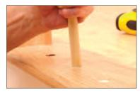
If need be, use an implement, such as the rod shown in the photo, to tap the dowel plug below the surface level.
