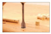
Previous hole size may vary, but are usually 3/4". If smaller, re-drill them with a 3/4" spade bit. If the holes are larger than 3/4", cut your own custom sized dowel to fit the hole.
